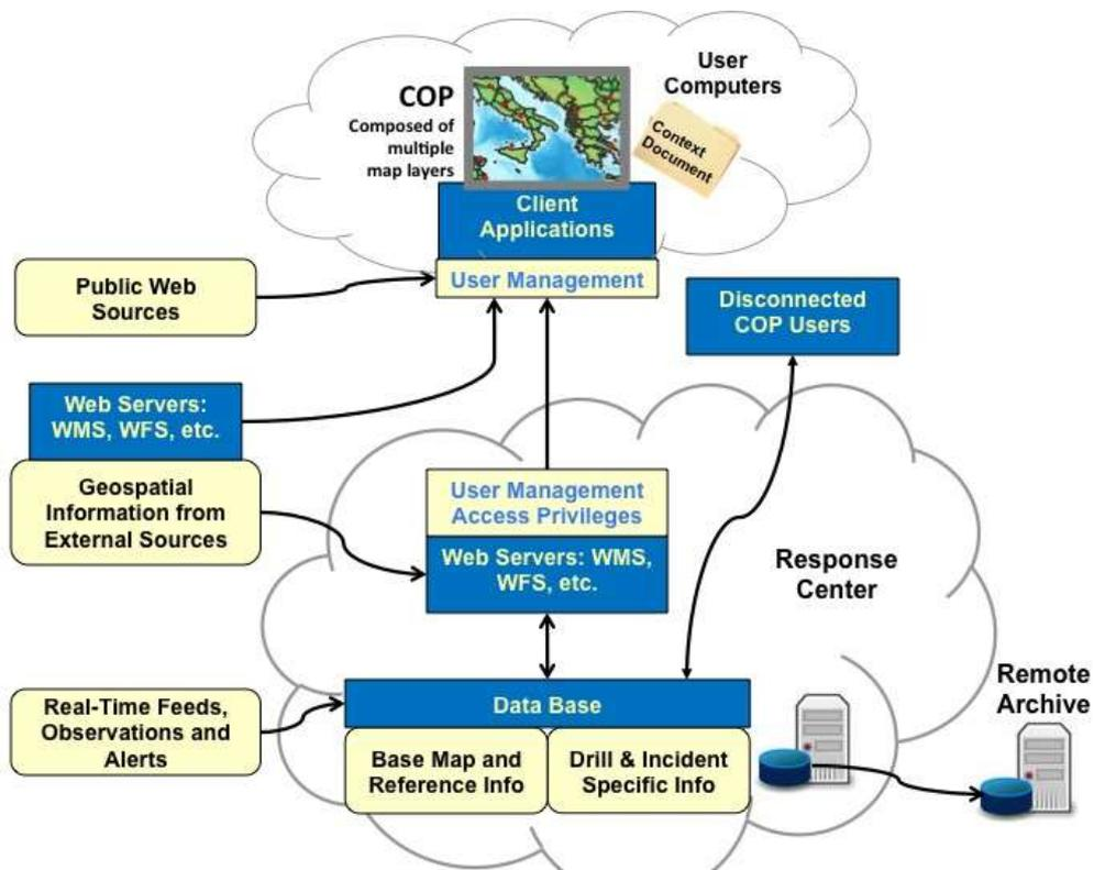
Figure 10: OSR Common Operating Picture (COP) delivery architecture
