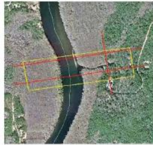
Limits of test area (lines crossing the project limits indicate flight paths for the LiDAR survey)
