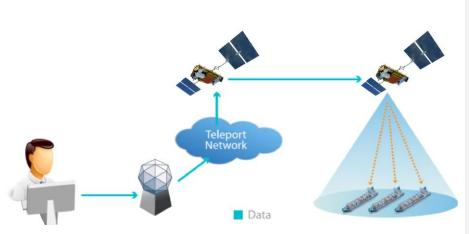
Figure 2 - Basic concept of the Iridium EGC system
