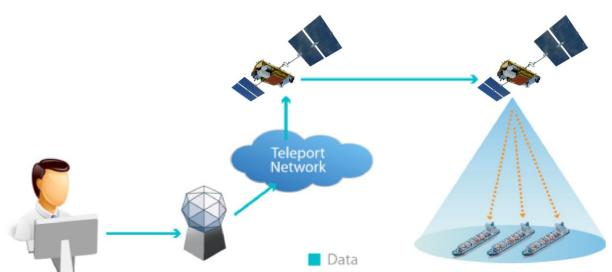
Figure 2 – Basic concept of the Iridium SafetyCast service
