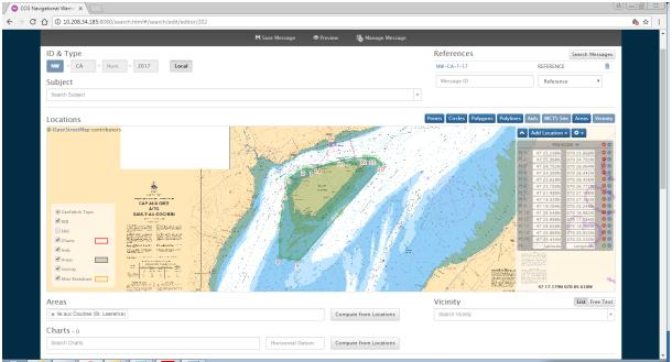
Figure 2 – User interface for creating NW, here an area NW.
