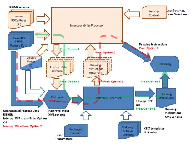
Figure 1. Interoperability Processing Overview for Phase 1
