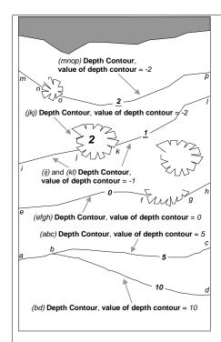
The boundary of a drying rocky area (see INT1 - J20) or coral reef (see INT1 - J22) may be coincident with the zero metre contour (see 'fg' in Figure). If it is required to encode this boundary, it must be done using the feature **Depth Contour** with the attribute **value of depth contour** = 0.
