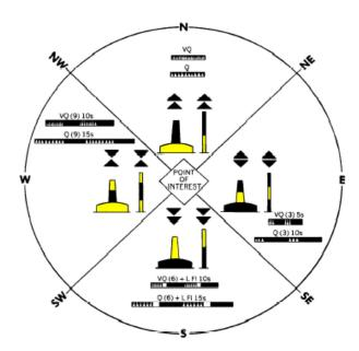
Lights, when fitted, are white . Very Quick Flashing or Quick Flashing; a South mark also has a Long Flash immediately following the quick flashes.
