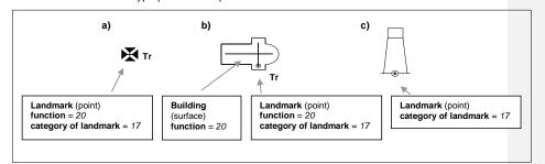
Not all landmarks are visually conspicuous. If a feature is visually conspicuous (that is, it is distinctly and noticeably visible from seaward), the attribute visually conspicuous must be encoded (see S-4 – B-340).
