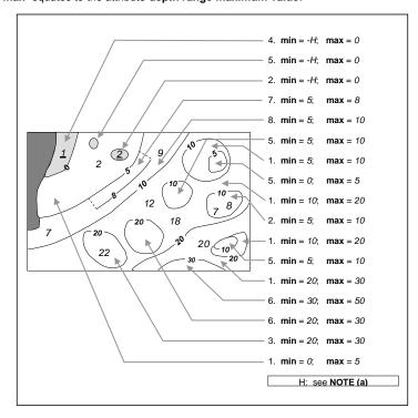
**NOTE (a)**: H = Height of the coastline datum above sounding datum, or a rounded value (for example (1) the value of the highest drying contour indicated on the source document; or (2) zero, if the coastline datum is the same as the sounding datum).
