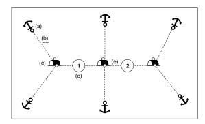
A complete mooring trot is composed of ground tackle, mooring cables, buoys and mooring berths on junction cables. The following remarks refer to the annotations in the Figure above:
