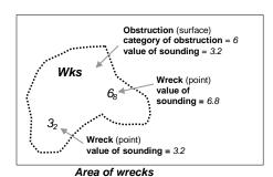
The area enclosed by the danger line must be encoded using **Wreck** (see clause **X.X**) or **Obstruction** (see clause **X.X**) features of type surface, with the attribute values, when encoded, reflecting the characteristics of the shallowest point feature encoded in the area. The area must also be covered by **Depth Area** or **Unsurveyed Area** features as appropriate.
