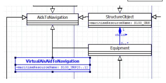
Figure 1 Addition of MRN to the structure- and VirtualAisAidToNavigation features.
