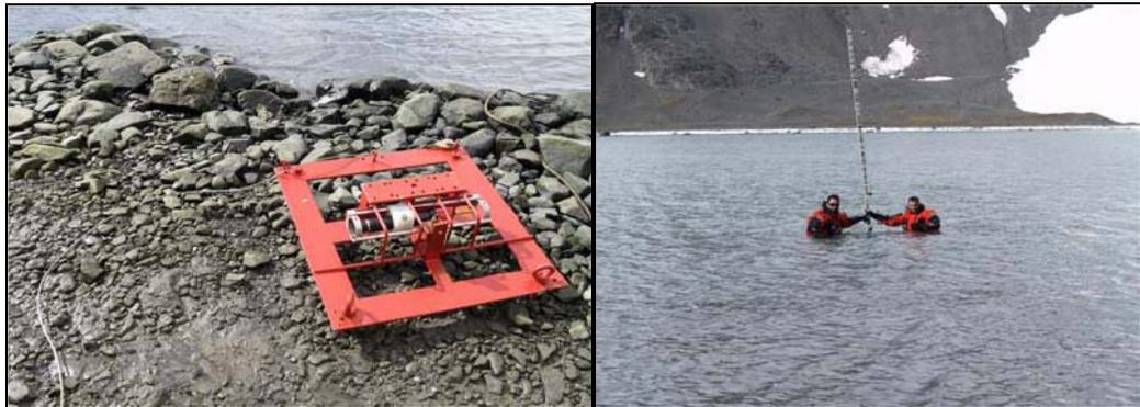
*Figure 10. Bottom pressure sensor for tide measuring*
