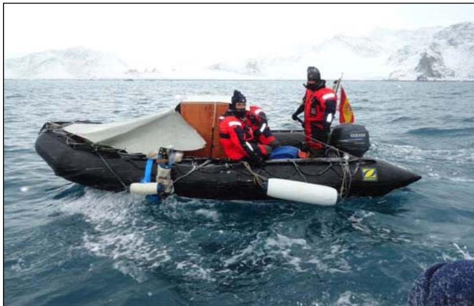
*Figure 7. Sounding with a shallow water portable multibeam sounder*
