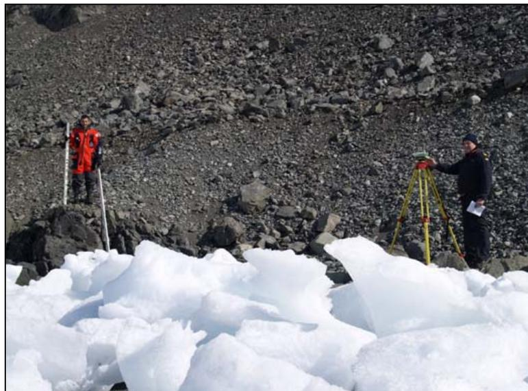
*Figure 11. Levelling tide bench marks*
