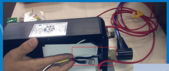
A defective RJ45 connector on the MB1 being repaired via remote assistance
