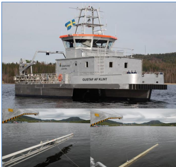
Figure 5 Bar sweeping survey vessel Gustaf af Klint. The bar is transverse across the stern and is here submerged into the water.
