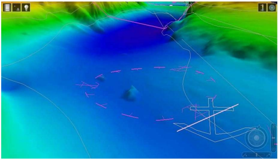
ENC data is created using CARIS' S-57 production tool. The bathymetric surface is created using CARIS BASE Editor.
