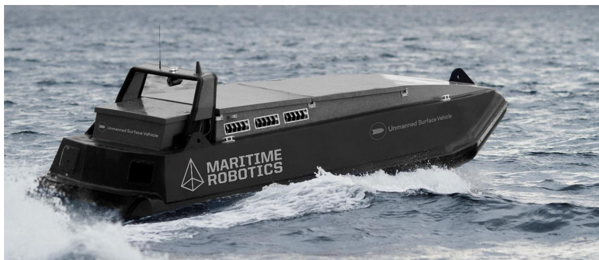
Fig. A new survey launch: Length 5.85m, breadth 2m, transit speed 30knots, 1 waterjet, MBES, and LIDAR.
