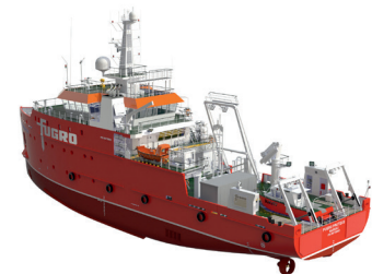
Backdeck layout and facilities allow fast mobilisation and flexibility of configuration.
