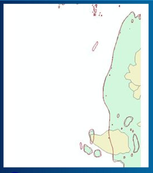
To make the derived depth contours more true-to-life, the SWIR extracted shoreline polyline verticies were converted to point, and added to the bathymetry as a depth value = zero
