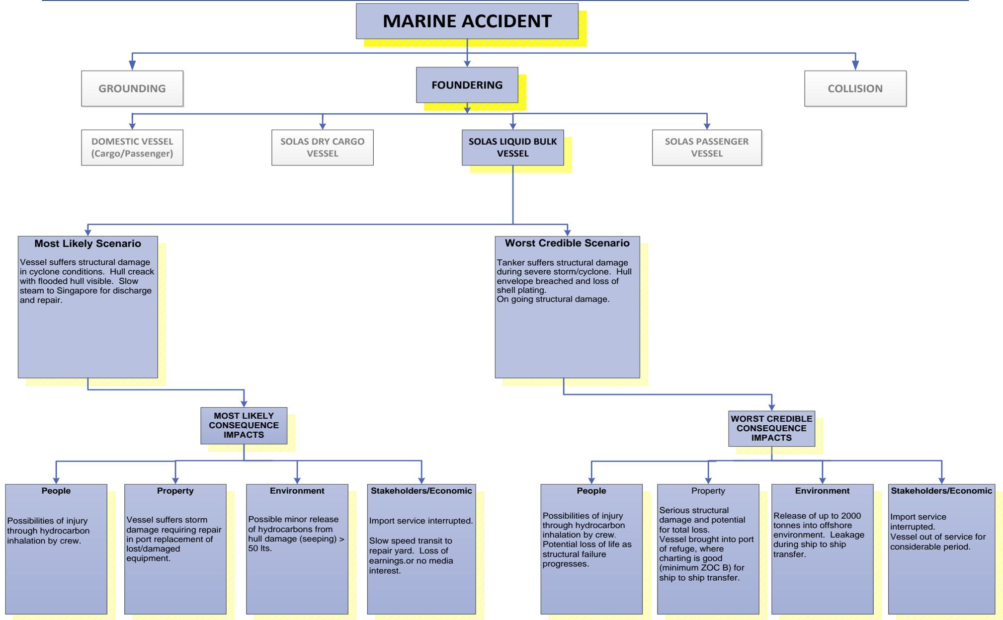
Figure 8: SOLAS Liquid Bulk Vessel Foundering Scenario
