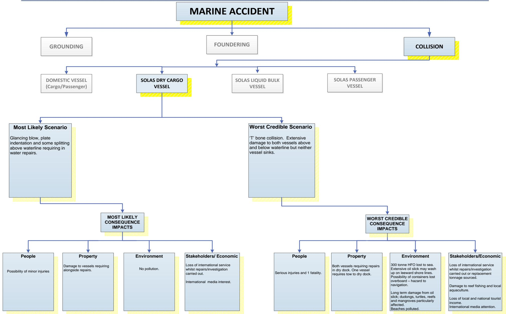
Figure 10: SOLAS Dry Cargo Vessel Collisions Scenario
