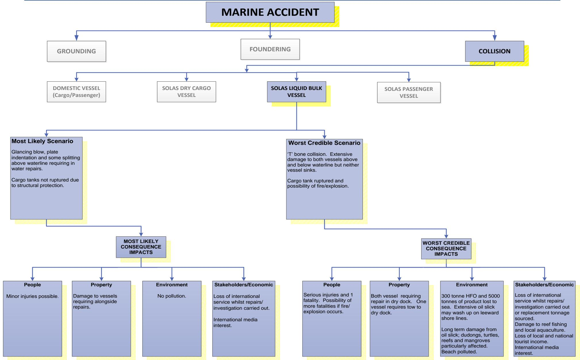
Figure 11: SOLAS Liquid Bulk Vessel Collisions Scenario
