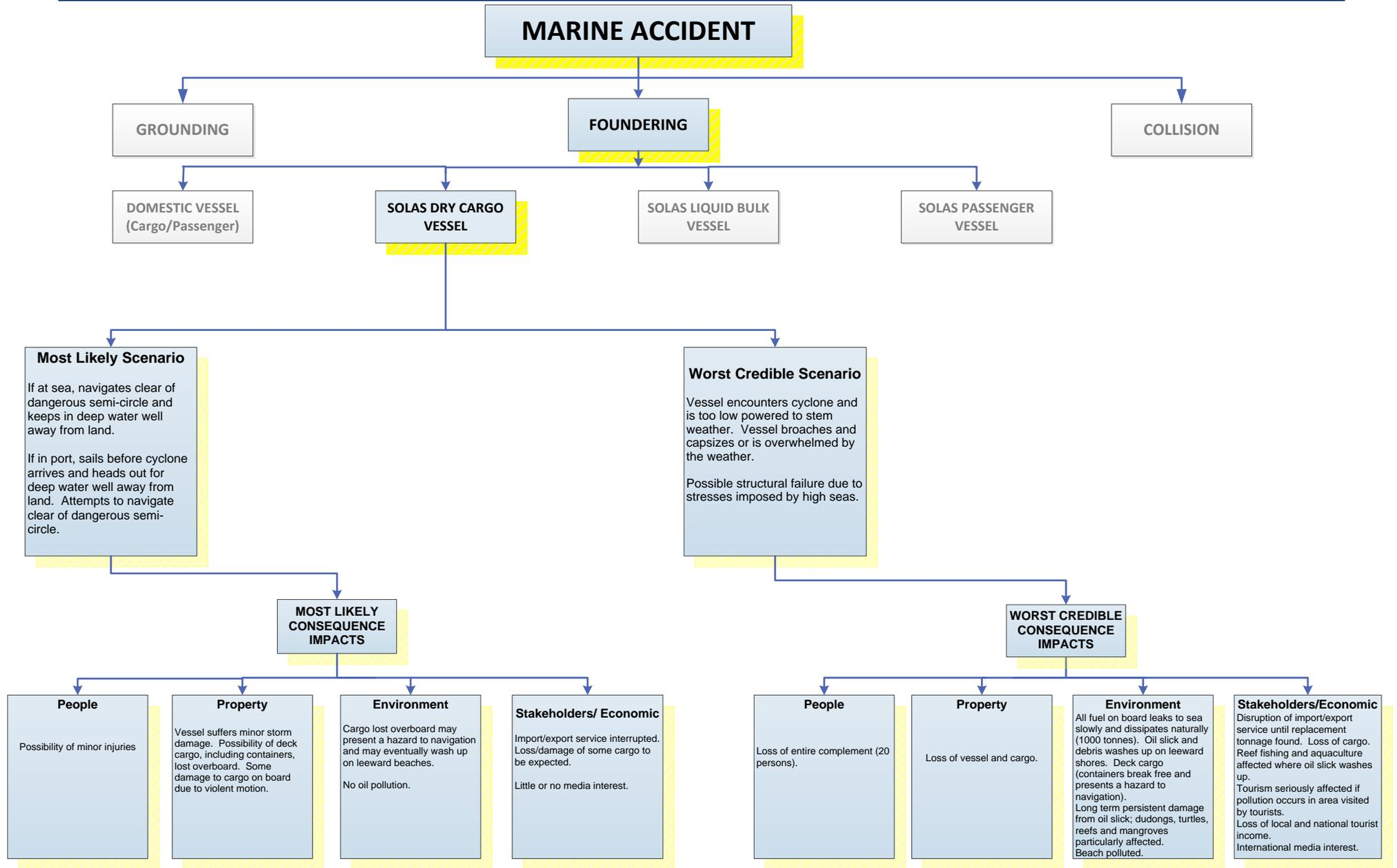
Figure 6: SOLAS Dry Cargo Vessel Foundering Scenario
