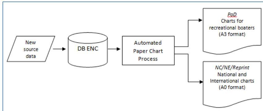
Fig.9. Combined ENC to paper nautical chart workflow
