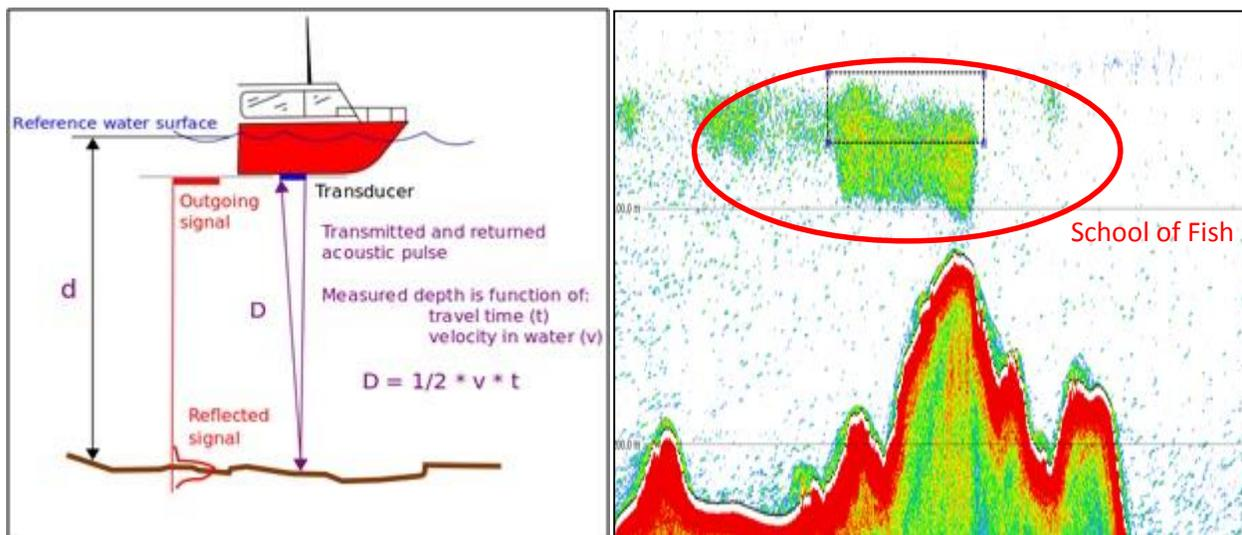
*Figure 7.* Example of estimating depth with a simple echo-sounder (left), and illustration (right) of the potential for blunders (e.g., the echo-sounder detecting the depth of a school of fish, rather than the seafloor).
