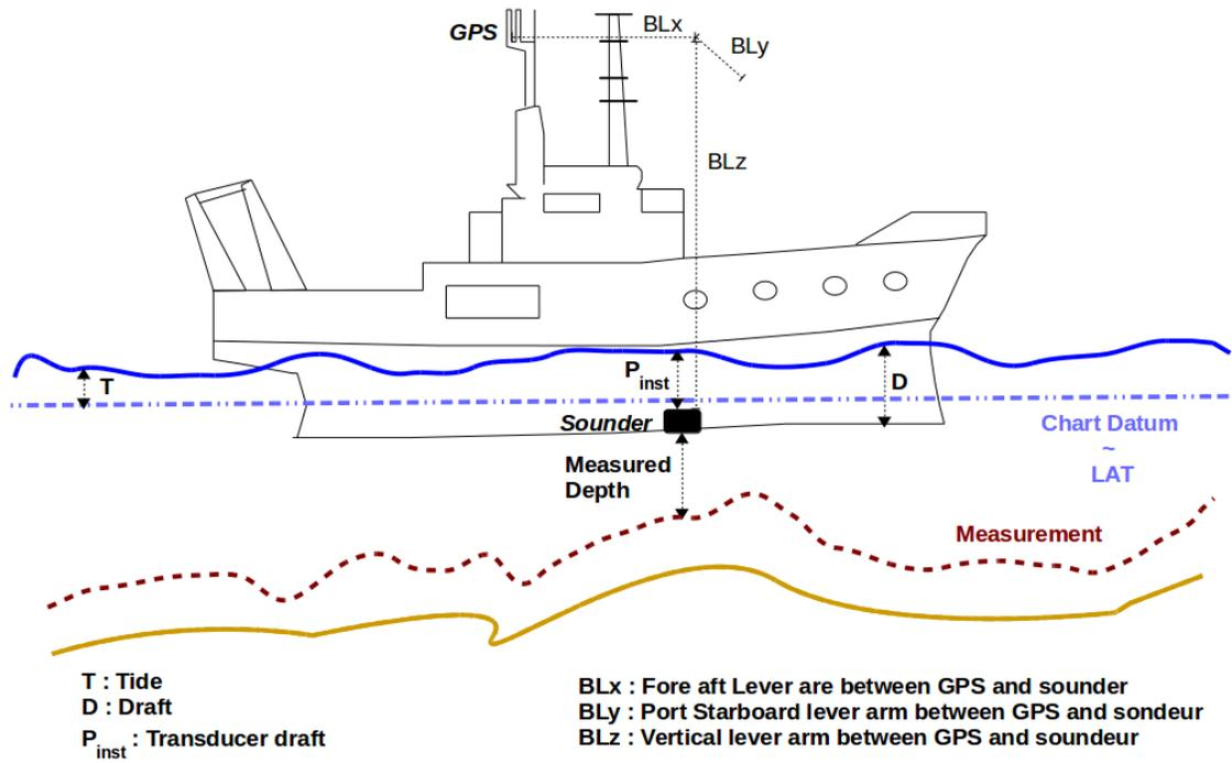
Figure 11. Examples of the effects of not correcting for vertical offsets. Here, not correcting for the offset of the transducer from the waterline leads to a measurement (red line) that differs significantly from reality (yellow line). This gives a bias (systematic) uncertainty to the measurements.
