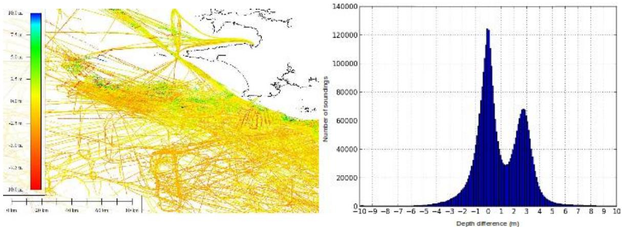
*Figure 14.* Difference between crowdsourced observations and a reference grid model (data courtesy of SHOM). Errors in the crowdsourced observations are clearly seen in plan view (left) and are reflected in the bimodal distribution of differences (right). The uncertainty associated with the crowdsourced observations might not reflect these differences if the observer’s metadata was incomplete.
