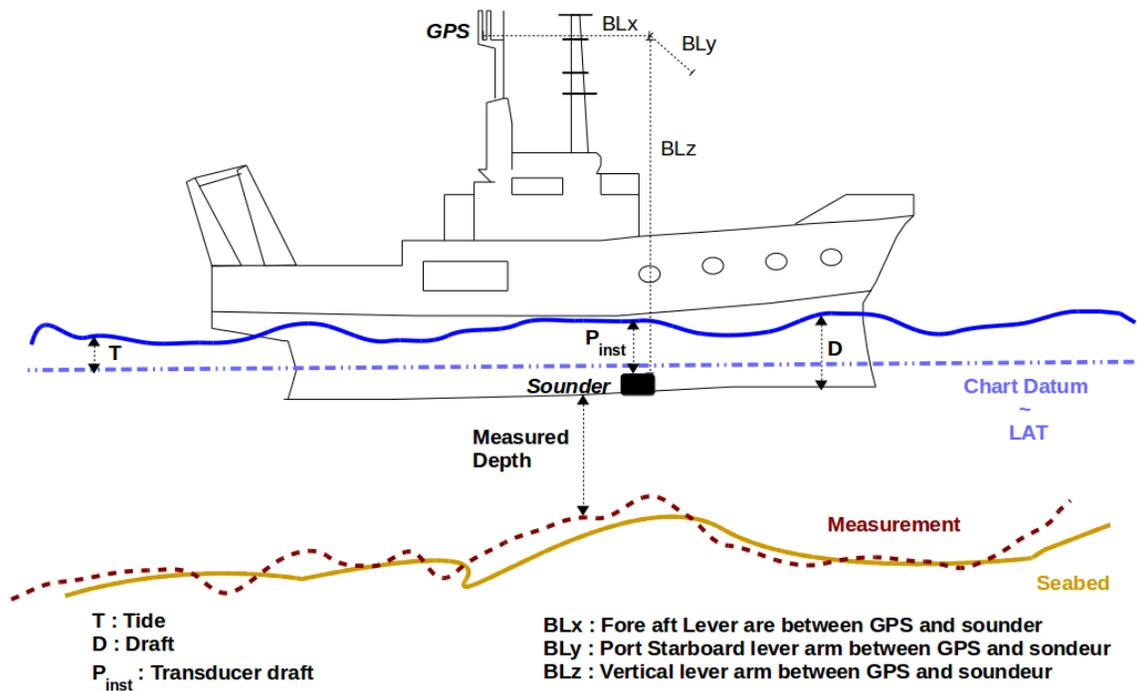
Figure 12. Effects of not correcting for horizontal offsets. Here, not measuring the horizontal offset between the GNSS receiver position and the echo-sounder results in along-track offsets of seafloor features. Red line: measured; yellow line: reality.
