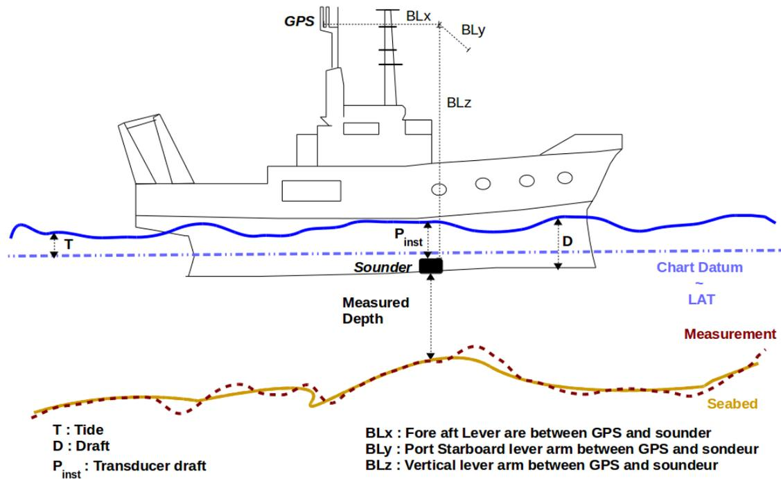
Figure 10. Effects of accurate, but not precise uncertainty on a depth sounding. Here, on average the depth measured (red line) is correct but point to point it varies from the true depth (yellow line).
