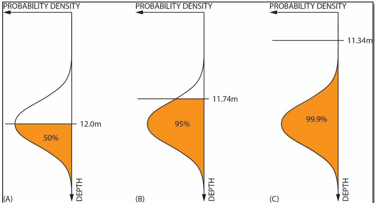
Figure 13. Examples of shoal-clearance depths for different probabilities of excession, based on the same basic uncertainty estimate of  $12.0 \pm 0.3\text{m}$  (95% CI). Assuming a 12.0m clearance is only true 50% of the time (left); a 5% probability of being shallower requires the depth to be reduced to 11.74m (middle); a 1:1000 chance of being shallower requires a clearance depth of 11.34m (right).
