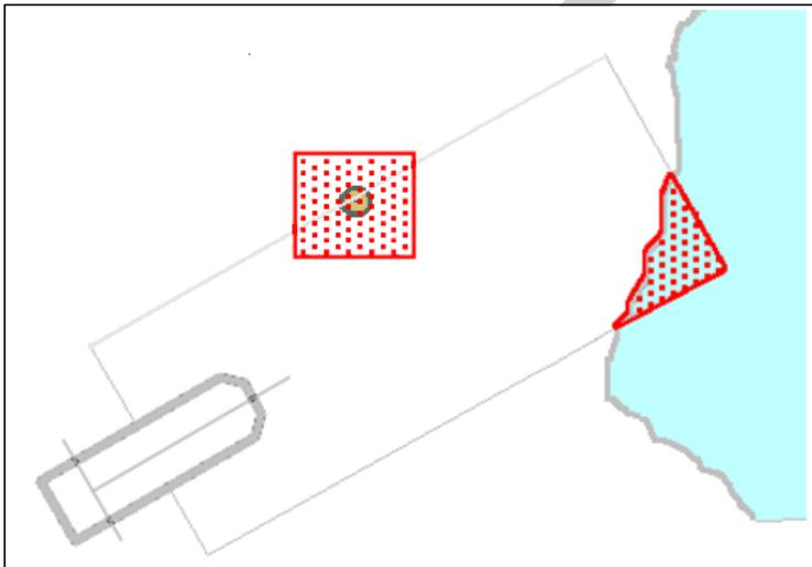
Fig 8. Example Danger Highlight in ECDIS
