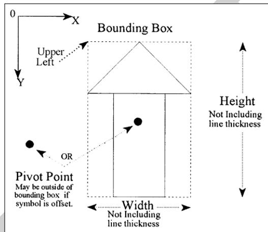
Fig 2. Pivot point, bounding box and symbol coordinates.
