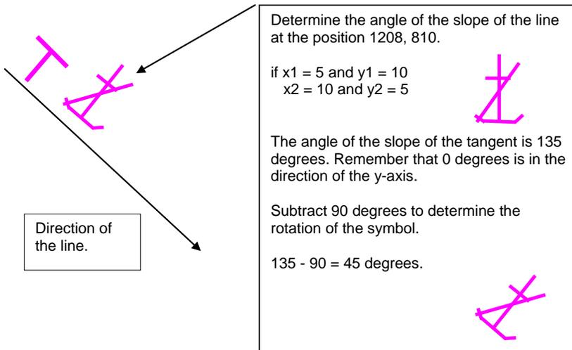
STEP 4: Repeat with the other straight line segments and the VLINEMAG symbols.
