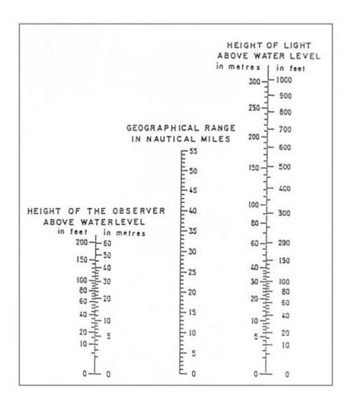
By using the above nomogram a geographical range can be determined by placing a straightedge against the height of the respective light and the height of the observer above water level.
