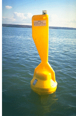
Wind measuring meteorological drifting buoy
