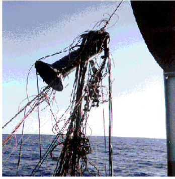
Longline fishing gear entangled in a TAO mooring.
