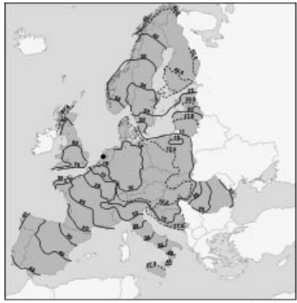
Figure 2: UELN 95/98 – Isolines of Precision
