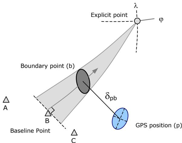
To compute the precision to which the user's position ( $p$ ) is determined with respect to a maritime boundary, we need the variance matrix of the vector  $\delta_{pb}$ . This variance matrix produces the *relative error ellipse*, which expresses the precision of point ( $b$ ) with respect to point ( $p$ ). Any errors common to the two points are removed as a result of their geometrical difference. Figure 5.2 illustrates the concept of the relative error ellipse.
