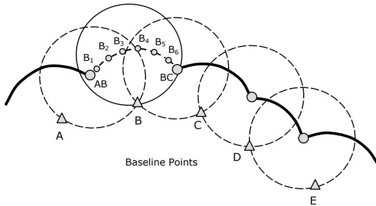
Figure 3.3. Construction from a Straight Baseline (Murphy et al., 1999)
