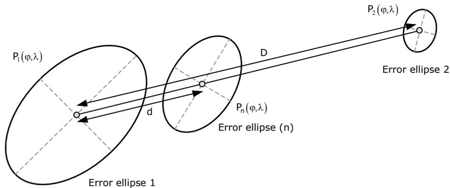
The variance matrix of point  $P_n$  can be computed using equation (2), where  $A$  is the matrix relating the random point  $P_n$  to points  $P_1$  and point  $P_2$ , and  $V$  is the variance matrix for points  $P_1$  and  $P_2$ .
