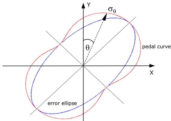
In Figure 4.1, the semi-major and semi-minor axes of the error ellipse represent the maximum and minimum precision in the position of the point to which the error ellipse applies. The pedal curve enables the precision of the point in any arbitrary direction  $\theta$  to be determined ( $\sigma_\theta$ ) (Cooper, 1974).
