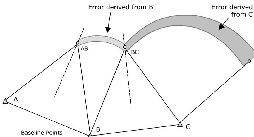
Figure 4.3. The propagation of error from a Straight Baseline
