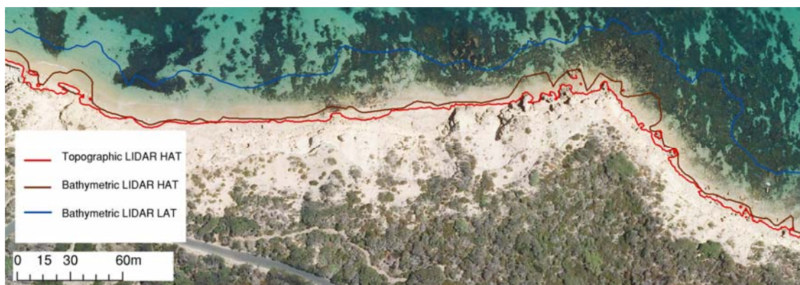
Figure 8 - Comparing HAT lines derived from bathymetric and topographic LIDAR - near Port Phillip Heads, Victoria
