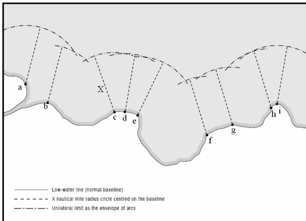
**Figure 2 Envelope of arc and relevant basepoints**
