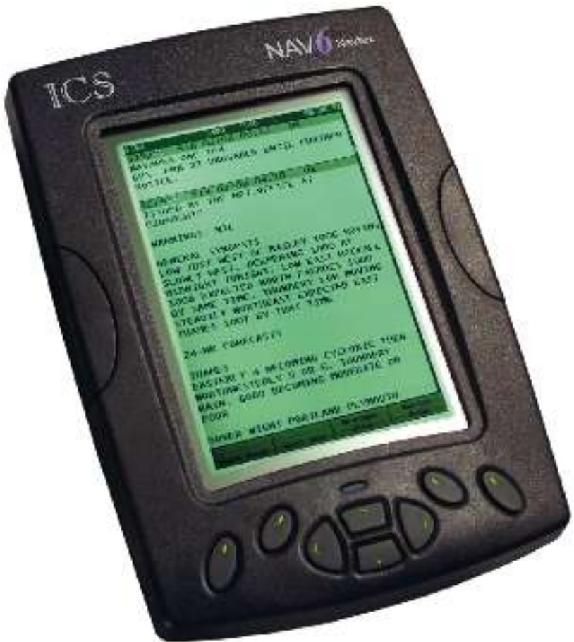
Figure 5 – Example of NAVTEX receiver with LCD screen
