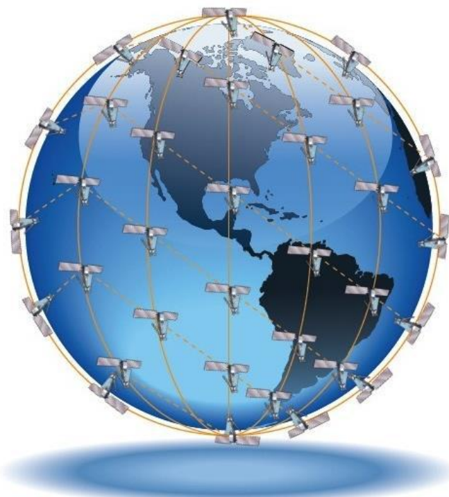
Figure 1. Schematic diagram of the Iridium constellation showing the six orbital planes.
