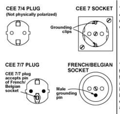
The CEE 7/4 plug has two 4.8mm round contacts on 19mm centers and two grounding clips on the sides of the plug body.
