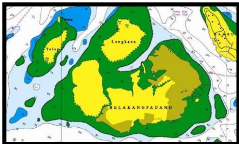
Pict.4. ID Chart no. 44 (1:25,000) shows houses/villages that exists along the coastline and on water is charted using a settlement symbol
