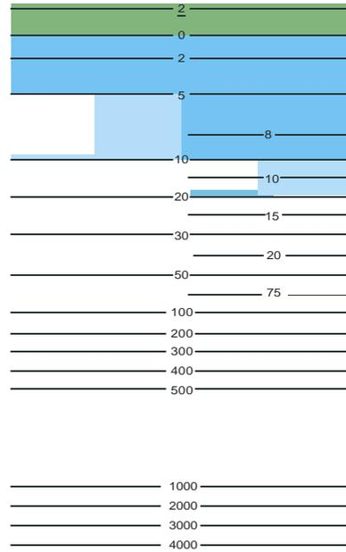
**Supplementary contours**, eg at 3, 8, 15, 25, 40, 75m and multiples of 10 or 100m may be shown, **if the available data permit, to delineate particular bathymetric features where soundings would otherwise be the only depth information over a large area, or for the benefit of particular categories of shipping. The 2500m contour may be required for measuring continental shelf limits (see UNCLOS Article 76)**
