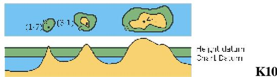
**B-421.2** **Rocks, boulders and rocky areas which cover and uncover** must be shown either by being outlined with the low water rock edge symbol (see B426.2), with intertidal tint superimposed, or, where **appropriate isolated**, by the symbol for a pinnacle \* . Drying heights must be shown above Chart Datum in the standard way (see B-413.1) and enclosed in brackets where out of position.
