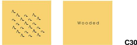
**B-354.2** Prominent trees when found in small groups (as opposed to stretches of woodland) may be represented by pictorial symbols. When the position of an individual isolated tree is known, and is of use in position-fixing, a small circle must be inserted at the base of the symbol.
