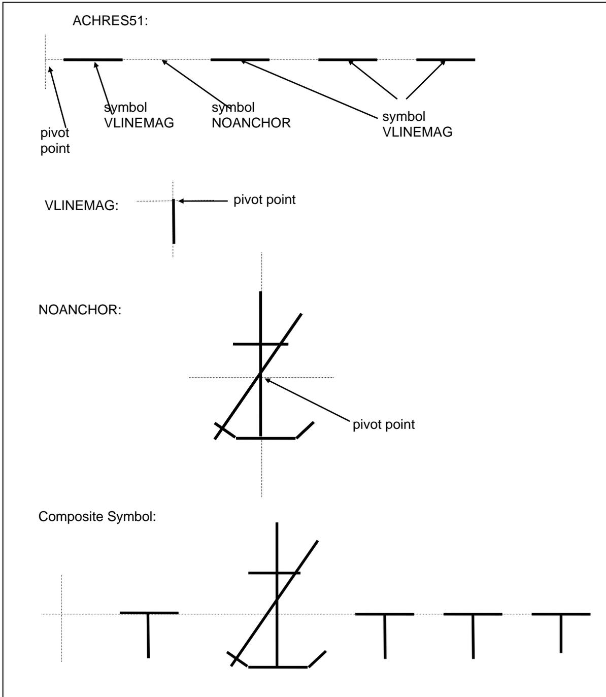
3. Re-number "Fig. 3-Usage of complex linestyle" as "Fig. 3a.-Usage of single unit type of complex linestyle", and add new "Fig 3b-Usage of composite type of complex linestyle" shown above
