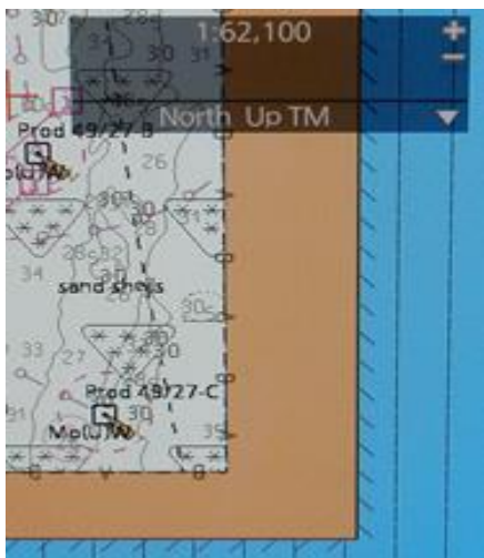
(Figure 18 - ECDIS D Differing overlap view based on display scale)
