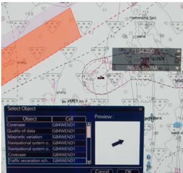
Figure 13 – ECDIS D displaying TSSLPT with multiple cells listed in Pick Report, GB4WEND1 selection highlighted
