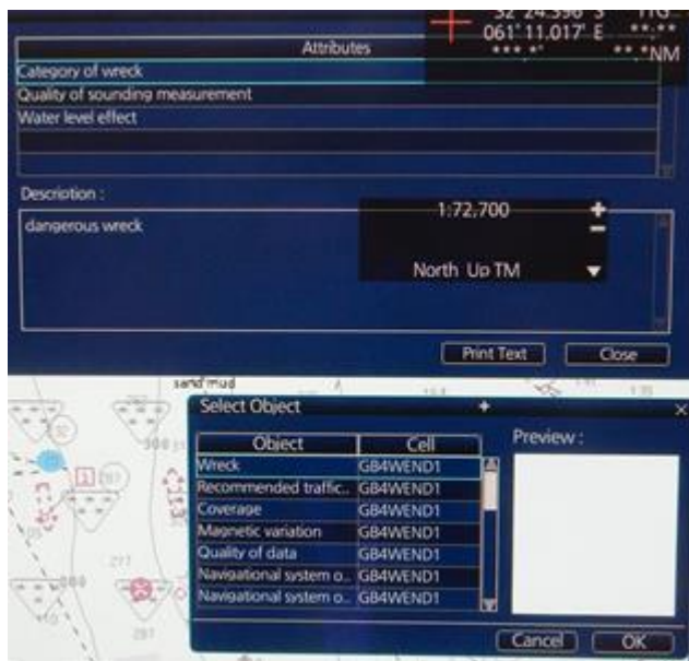
Figure 15 – ECDIS D displaying GB4WEND1 WRECKS with dangerous wreck attribution
