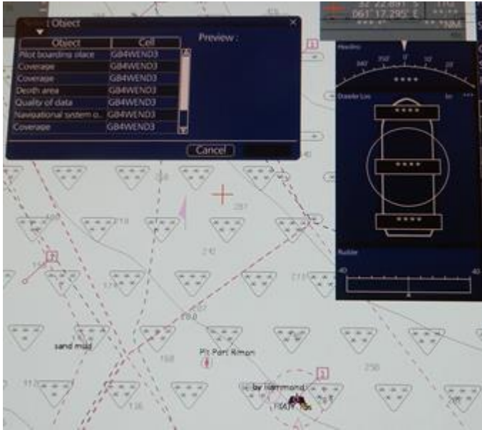
Figure 19 – ECDIS D GB4WEND3 displaying at 43k with PILBOP visible
