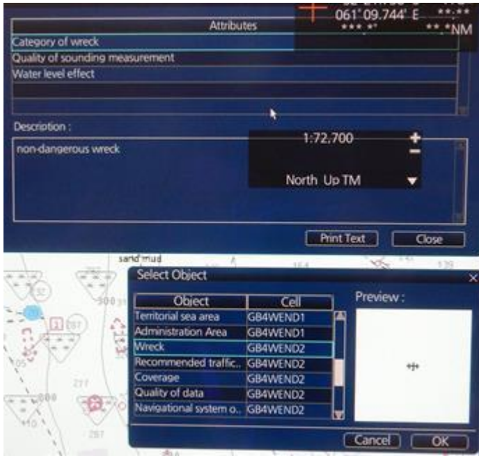
Figure 16 – ECDIS D displaying GB4WEND2 WRECKS with dangerous wreck attribution
