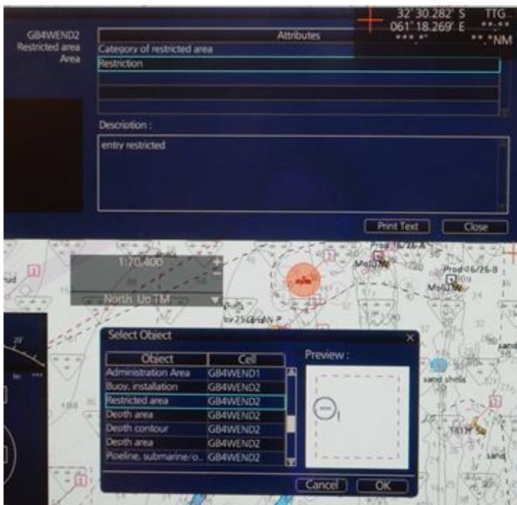
Figure 11 – ECDIS D displaying RESARE with multiple cells listed in Pick Report. GB4WEND2 displays entry restricted
