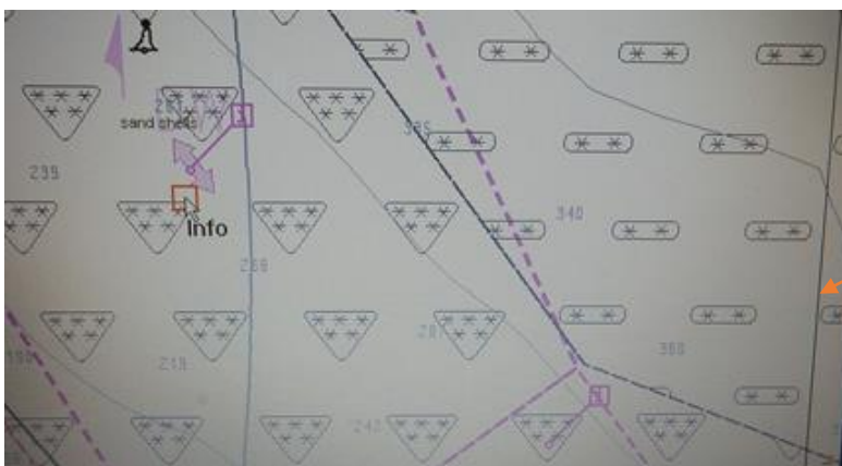
Figure 6 - On ECDIS C the orange info point picks up GB4WEND2 as the edge of GB4WEND1 enters the screen.
