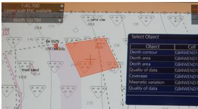
Figure 7 - TSSLPT highlighted on ECDIS D at 45k
