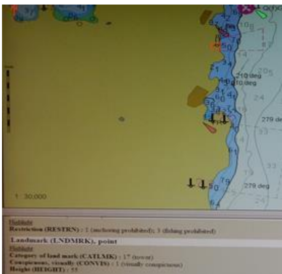
Figure A10 – LNDMRK (convis) displaying on GB4WEND3
