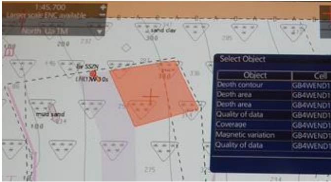
Figure D10 - TSSLPT highlighted on ECDIS D at 45k
