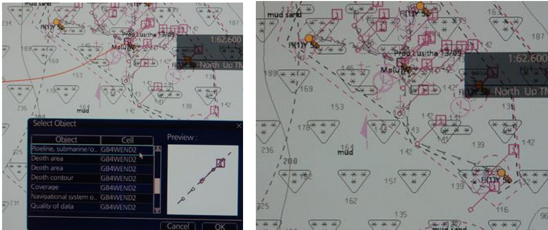
Figure D16 – PIPSOL can be highlighted from the Pick report but doesn't display on the cell
