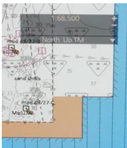
Figure D5 – GB4WEND1 & GB4WEND2 Differing overlap view based on display scale
