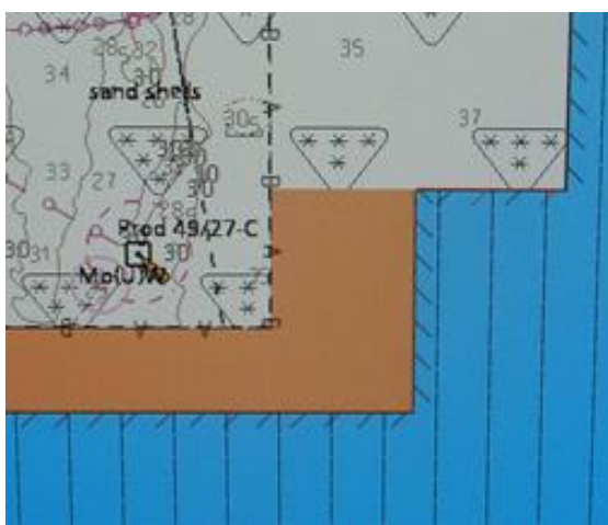
Figure D7 – ECDIS D displaying M_COVR as land tint
