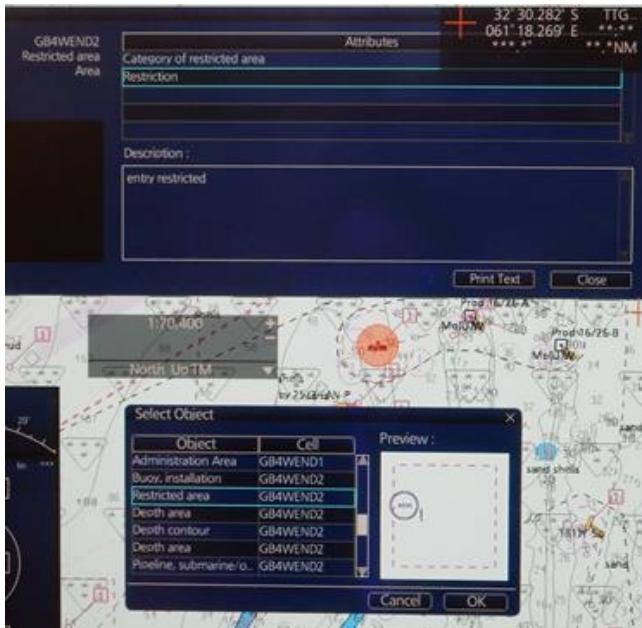
Figure D13 – ECDIS D displaying RESARE with multiple cells listed in Pick Report. GB4WEND2 displays entry restricted
