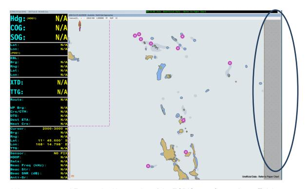
AU130150, panned Eastward, with a section of the ECDIS manufacturer's unofficial background world map visible (highlighted). This unofficial data invokes the "Unofficial Data –Refer to Paper Chart" message in the lower right corner of the screen.
