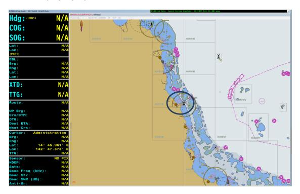
AU220140 with a Geotiff of Aus262 loaded however, due to the current zoom level the geotiff is only being shown as a chart outline (highlighted). This chart outline still invokes the smaller "Unofficial" warning upper left corner of the screen only.
