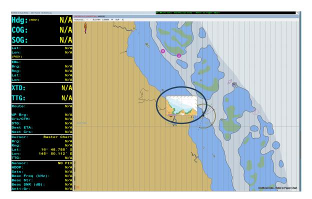
AU220140 with a Geotiff of Aus262 loaded and due to the increased zoom level the geotiff is now visible overlayed on the ENC. This invokes unofficial data warnings at **both** upper left and lower right of the screen.
