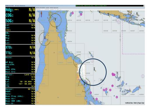
AU130120 with an overlay of Geotiff\* of Aus831 (highlighted). The Geotiff overlay invokes the "Unofficial Data –Refer to Paper Chart" message in the lower right corner of the screen. (\* Geotiff are scanned images of paper charts that are not suitable for navigation.)
