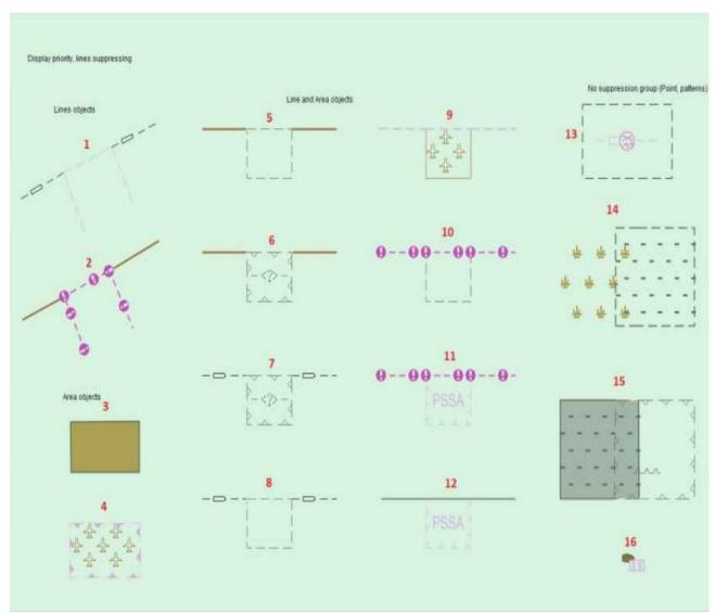
Object No. 2: When the radar is on, this picture is erroneous: here FORSTC (display priority 4, Overradar) and NEWOBJ (display priority 6, Subradar) have a common edge.
