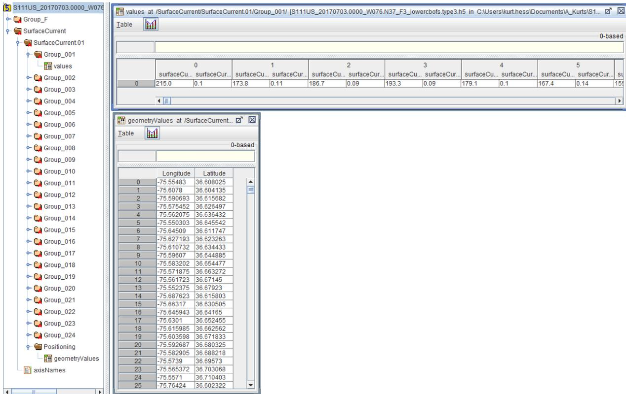
Figure G.8 – Image showing (left side) the structure of the file, and (right side) the one-dimensional compound array of values for ungeorectified gridded data (top panel) and the data in the group Positioning (bottom panel).
