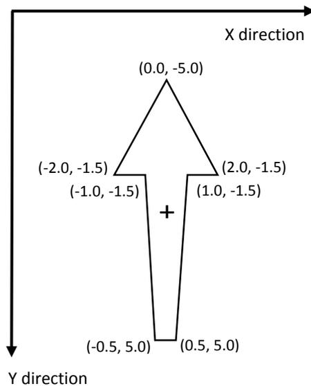
Figure 9.1 – Standard arrow symbol for use in representing surface currents. The coordinates of the vertices (x, y) are shown in mm. The '+' shows the location of the pivot point at (0.0, 0.0) and the y axis is pointing downward. Maximum height is 10 mm and maximum width is 4 mm.
