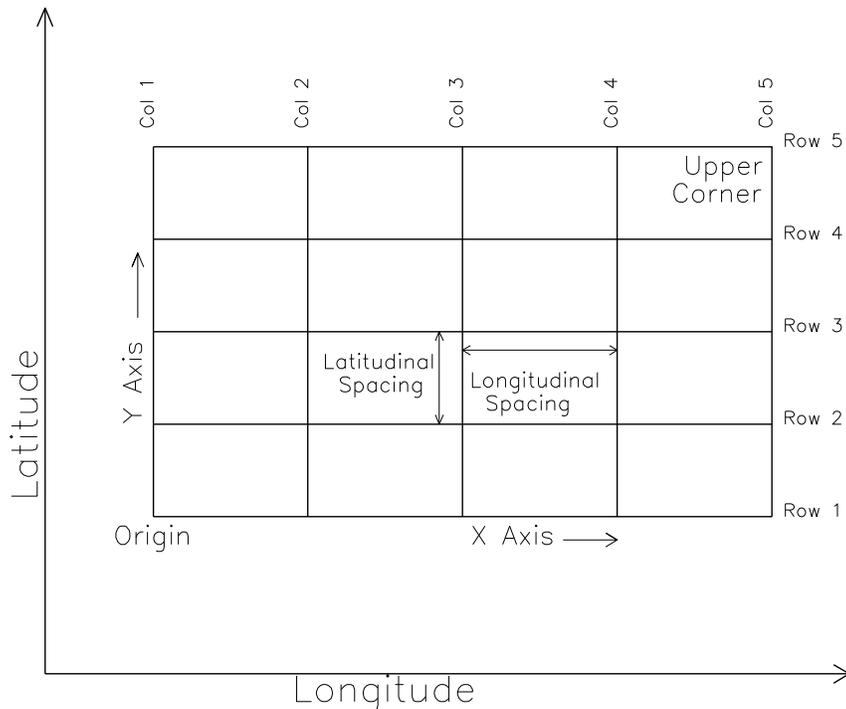
Figure 4.2 – Schematic of the regular grid and some of its attributes. The *offsetVectors* are shown as the Latitudinal Spacing and Longitudinal Spacing. The *origin* is shown at the lower left corner of the grid.
