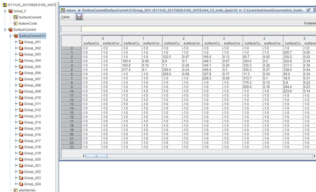
Figure G.5 – Image showing (left side) the structure of the file and (right side) the two-dimensional compound array of values for regularly gridded data.
