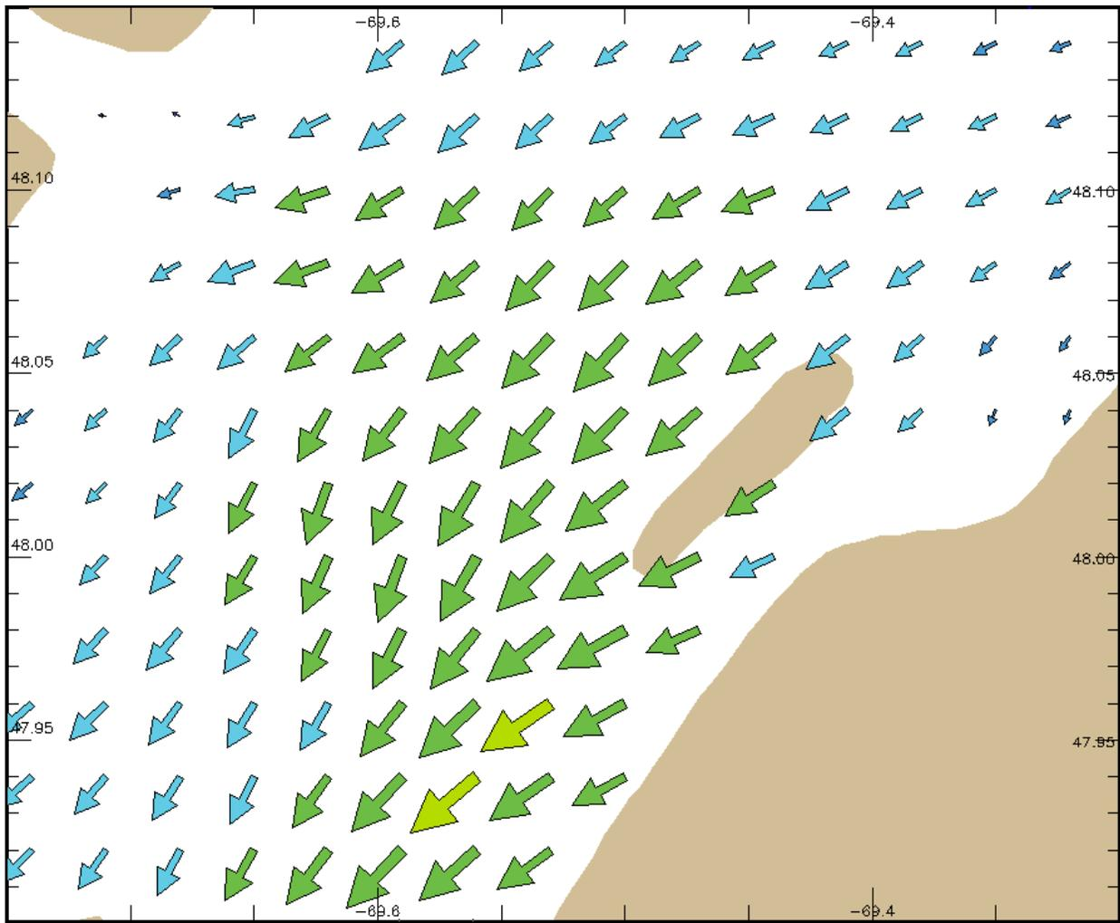
Figure 9.5 - Arrows representing gridded surface current data, with length increasing with speed, and  $S_{ref}$  is 5 kn,  $H_{ref}$  is 20 mm, and the maximum speed in the data in the image is 3.15 kn. Coastline added for clarity. Note that although some portions of the arrow symbol lie over land, the pivot point does not.
