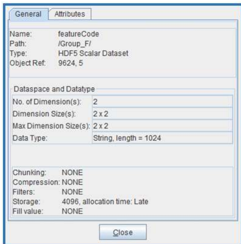
Figure B.3 - S-102 Group_F/featureCode Encoding general structure.
