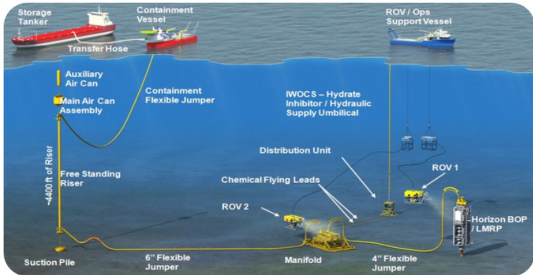
**Figure 1 Typical subsea well intervention project**
