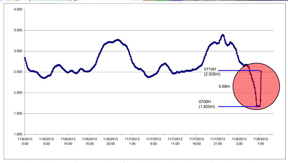
\* Actual observation transmitted/recorded based on the 10-minute interval, 1.820m at 0700H and last recorded data is 2.505m at 0710H above zero of tide staff. The tide house was damaged during the passage of the typhoon.
