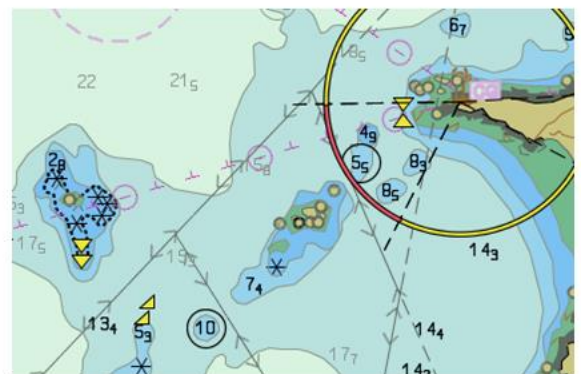
ENC displayed at 1 : 45 000 - No text displayed Overlap between objects (LNDARE, UWTRC)
