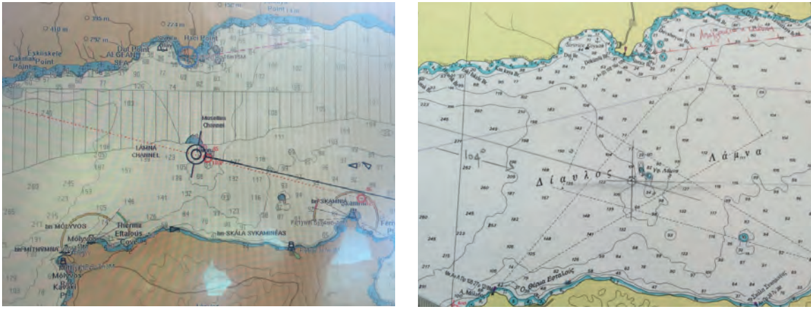
Figure 14: Left: Sector lights in ECDIS, right: sector lights on the Greek paper nautical chart. Source Dutch Safety Board
