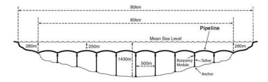
Sub-surface pipelines must be shown, where required, using the appropriate pipeline symbol as specified in clauses B-444.1 and B-444.2 above. To indicate the minimum design depth of the pipeline, a legend similar to *Water (submerged 250m – see Note)* must be placed along the pipeline, repeated as required if the pipeline extends across a substantial area of the chart. A cautionary note should be charted, for example:
