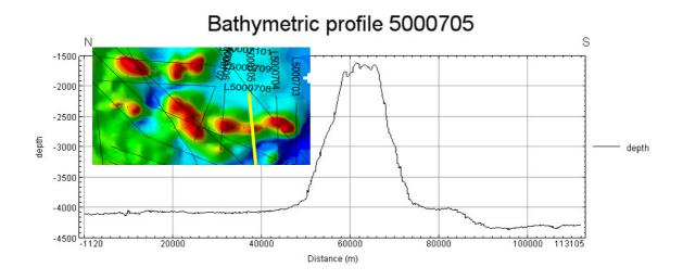
These Cruises were carried out by LEPLAC – The continental shelf survey during 1991-1992 years and were acquired by Almirante Câmara ship. The navigation systems used were Transit/GPS/Sonnar Doppler. The Bathymetric data were acquired employing echosounders suitable for deep waters.
