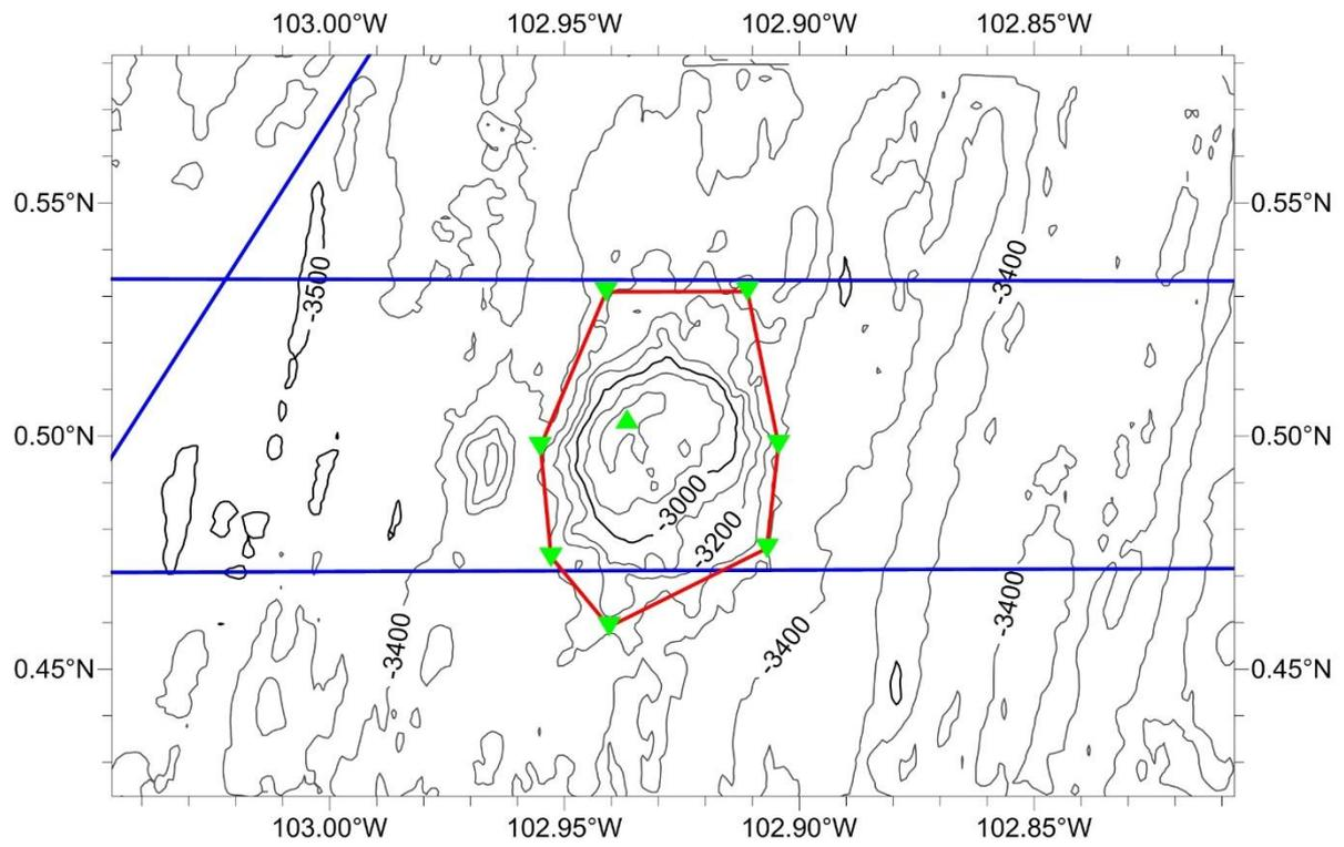
Fig 3. Isobath and survey line map of Baihua Hill (Contours are in 100 m, blue lines are survey lines)
