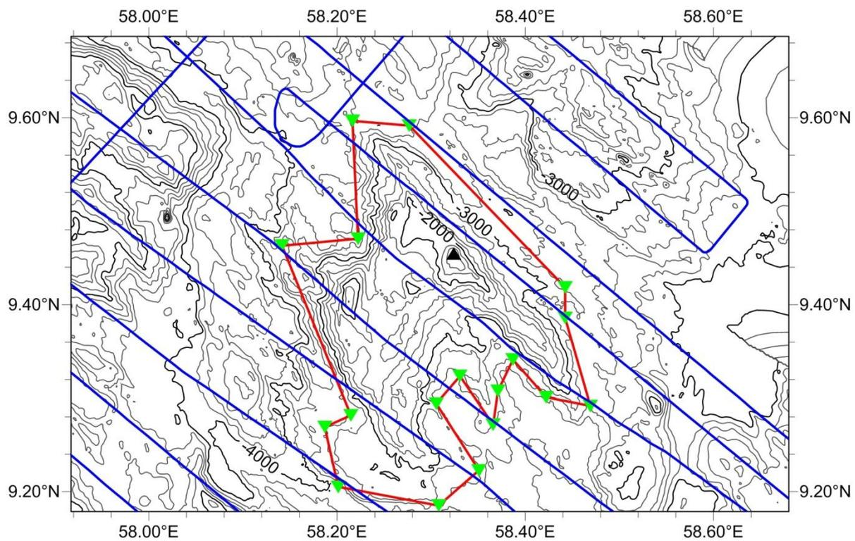
Fig 3. Isobath and survey line map of Wanwu Seamount (Contours are in 200 m, blue lines are survey lines)
