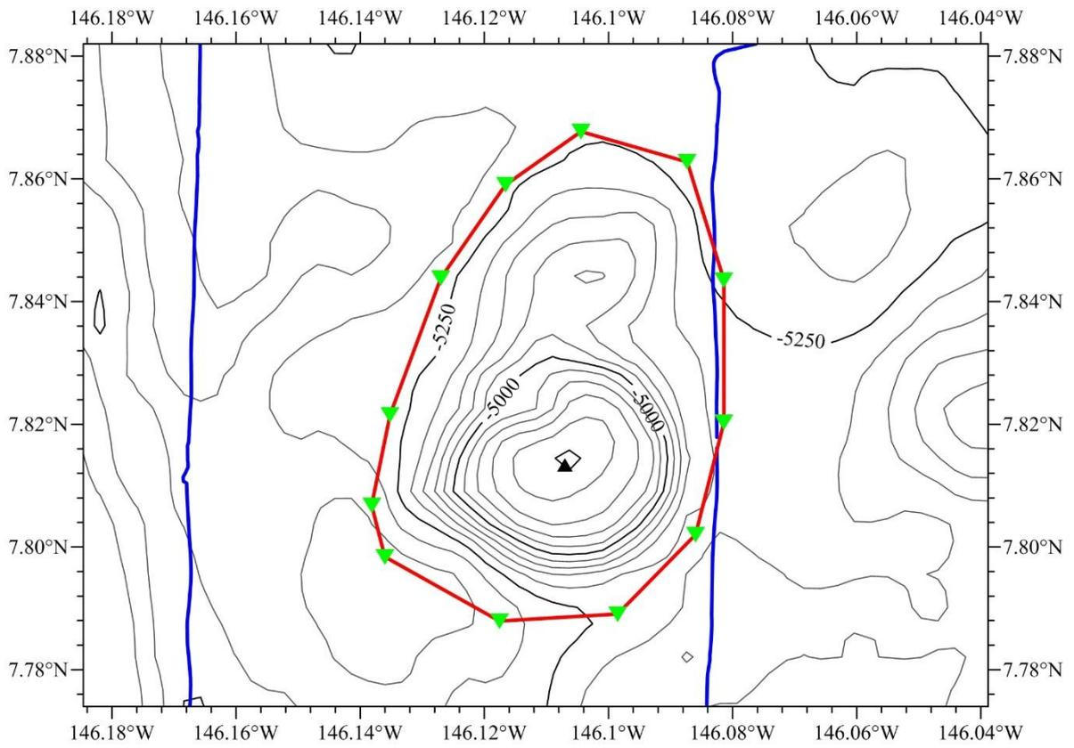
Fig 3. Isobath and survey line map of Wangbo Knoll (Contours are in 50 m, blue lines are survey lines)
