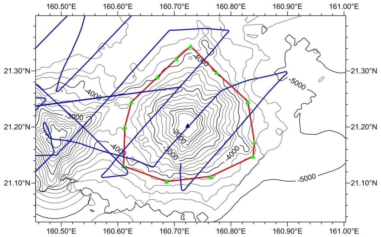
Fig 3. Isobath and survey line map of Baihe Guyot (Contours are in 50 m, blue lines are survey lines)
