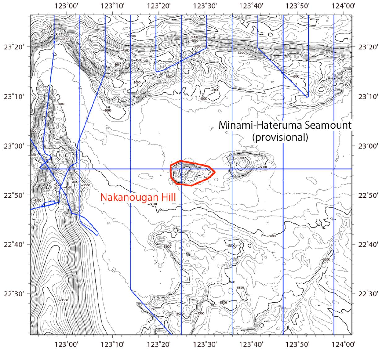
Fig. 2. Bathymetric map of the Nakanougan Hill, shown with track lines. Contours are in 100 m.
