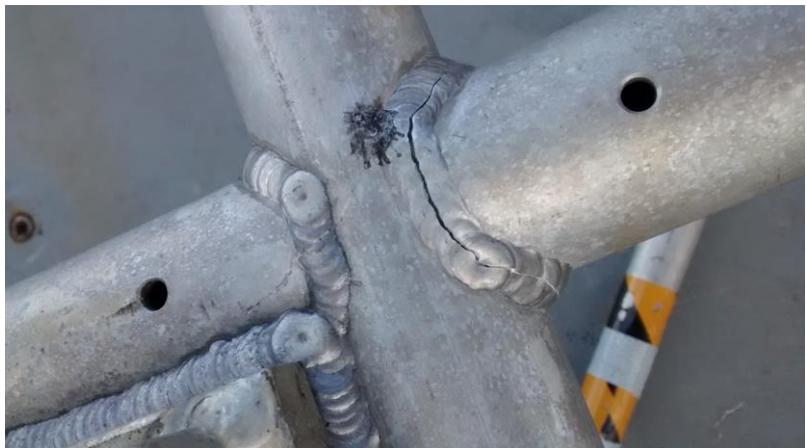
**Above:** One of the fractures sustained during a bad weather recovery. These were also fixed by *Falkor*'s engineering team
